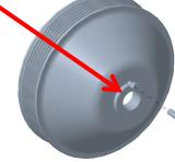
Rotate the OE belt tensioner CCW and remove the belt from the power steering pulley only. This is to remove tension from the belt temporarily. This belt will be reinstalled.
